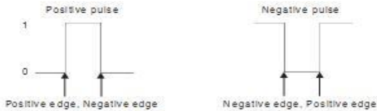
Figure 7.46 Clock pulse transition.
