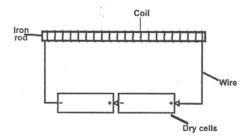
Which of the following energy transformations occur in the electromagnet?
